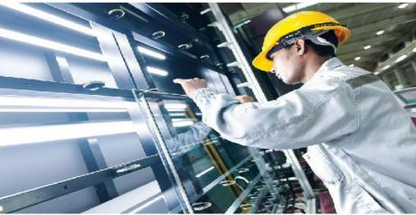
Sealing: Aluminum spacer is automatically curved and formed with the fewest joints and dual seals are applied, which ensures excellent sealing characteristics and long application lifetime
